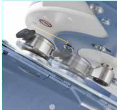
Pedal radius length adjustment
